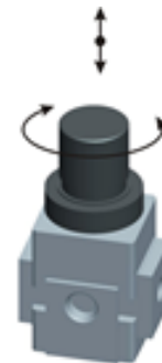
Fig. 15: Setting outlet air pressure
